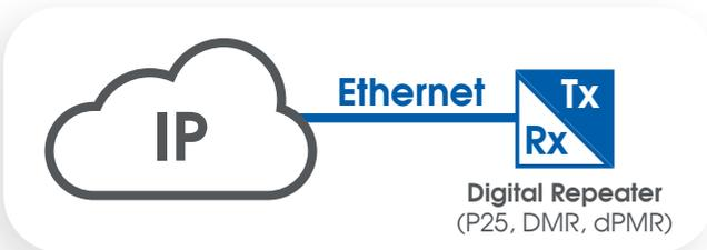
Where an IP connection is available, setting up and connecting to a radio network is quick and easy. In this case the term “digital repeater” is used as a generic term for any digital format such as P25, DMR or dPMR (NexEdge).
