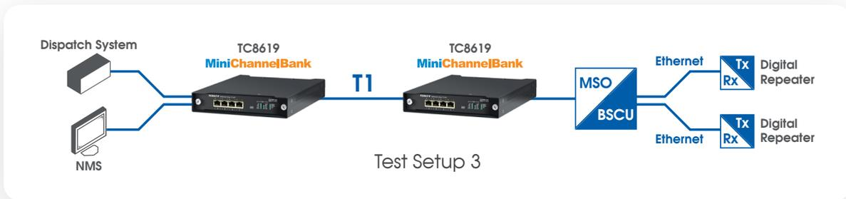
Once again, as soon as the system was connected it operated perfectly. There were no link alarms and the links were well within the required parameters. Multiple calls from the dispatcher were setup and again there was no increase in digital delay across the system.
