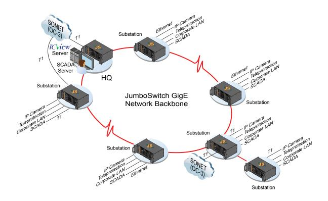
The Utility used the JumboSwitch network for a wide variety of applications including substation, SCADA, Teleprotection, Automatic Meter Reading (AMR), telecommunications, data services (including rate control), security cameras, and office LAN traffic.
