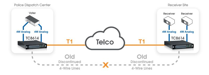
Above: The town replaced discontinued 4-wire leased lines with T1 lines from the Telco. Plug-and-play TC8614 devices convert 4-wire analog to T1. Dispatch equipment for the town remains the same.
