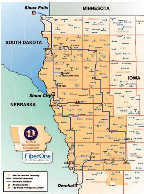
*NIPCO's fiber optic network consists of dual (redundant) fiber rings circling both the north and south ends of the NIPCO electric transmission system. The longest network ring segment between switches is about 40 miles (64km) and the shortest segment is 8.75 miles (14.4km).*
