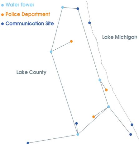
Above: ESRN replaced their leased lines with 4 and 2 wire cards. They integrated PTP 650 radios, a 4.9 GHz public safety network, and an OSPF network.
