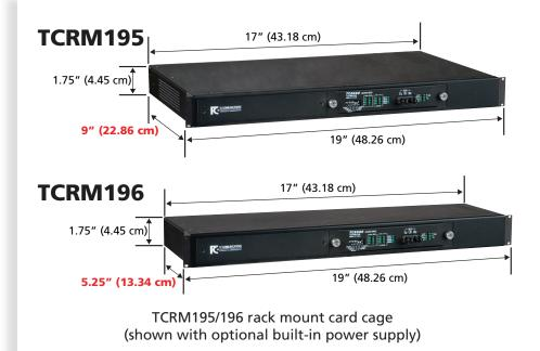
The TCRM195 and TCRM196 Universal Rack Mount Card Cages hold up to two single multiplexer or modem-type cards, or one doublemux or double-modem type card. In general the TCRM195 is used for multiplexers and the TCRM196 for modems.
