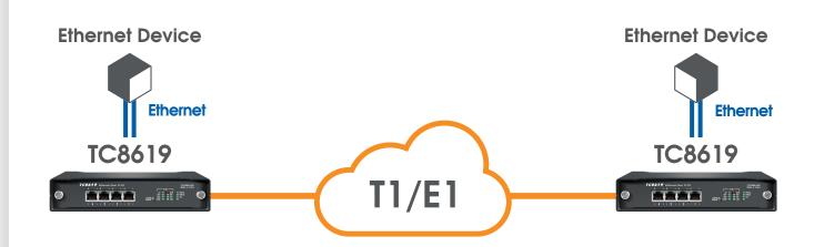
Typical Application using TC8619 Ethernet-over-T1/E1 Multiplexer
