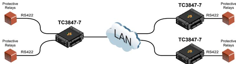
Typical "Serial Tunneling" Application Using TC3847-7 RS-422
