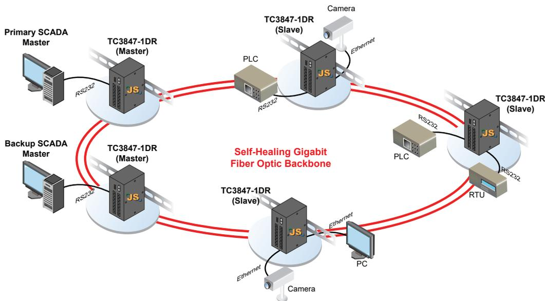
Typical Application using the TC3847-1DR in a Gigabit Ethernet Ring Network utilizing Dual Masters
