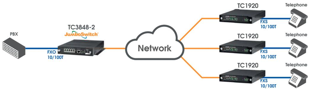
**Figure 1-3 Typical Application Using TC1920s to Extend Telephone Service via an Ethernet Network in a Substation Environment**
