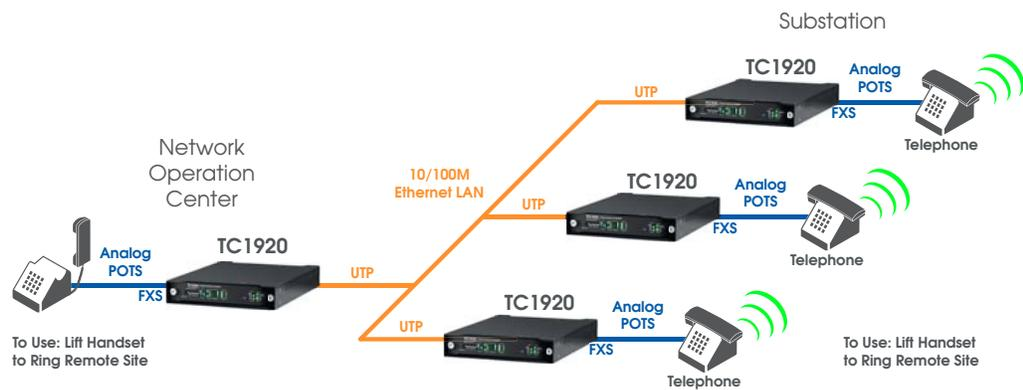
**Figure 1-4 Typical Application Using TC1920s to Provide Hotlink Service to Multiple Remote Locations**
