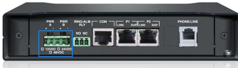
**Figure 5-3 TC1920 Back Panel Connectors and Indicators**
