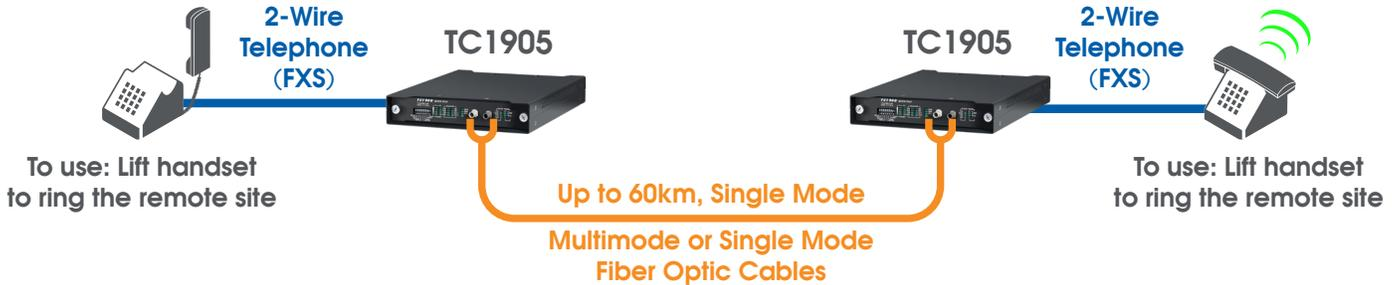
Typical Application Using TC1905s to Establish a "Hot Link" via One Fiber
