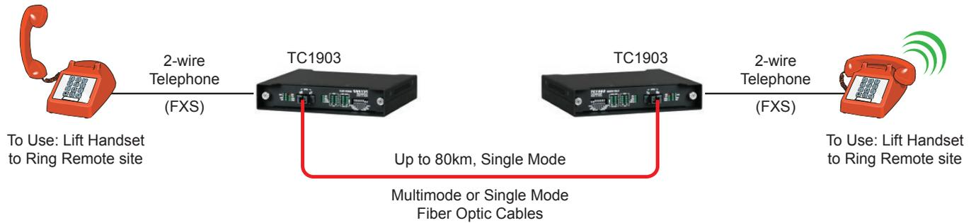
Typical Application Using TC1903s to Establish a "Hot Link" via Fiber Optic Cables
