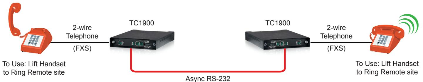
Typical Application Using TC1900s to Establish a "Hot Link" via RS-232
