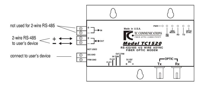
**CLK1, CLK2** - There are four DIP switches located on the same side of power supply terminals. The first two switches marked as "CLK1," "CLK2" are for RS-485's transition time setup. If both switches are at "up" position, then "IN" and "OUT" terminals are setup to RS-422's applications. If both or any of "CLK1" and "CLK2" is set to "down" position the electrical interface is set to RS-485 applications.
