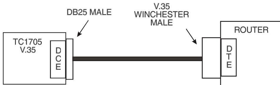
Figure 12. DB25 to V.35 Winchester DCE Pin Assignments
