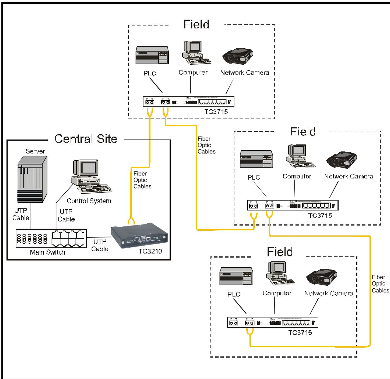
Figure 3. Daisy-Chain Diagram Using the TC3715's
