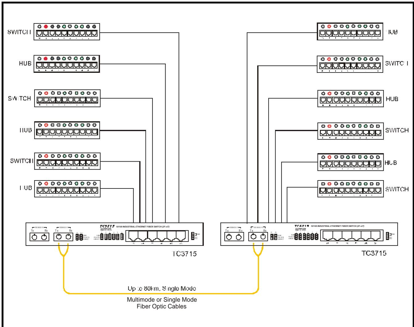
Figure 4. Backbone Using an Extended Star Topology with the TC3715's
