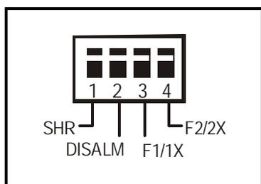
**Figure 6.** Front Panel Dip Switch
