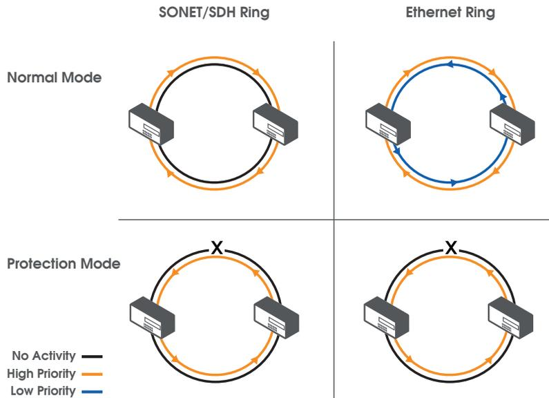
Figure 3: Protection Bandwidth Comparison
