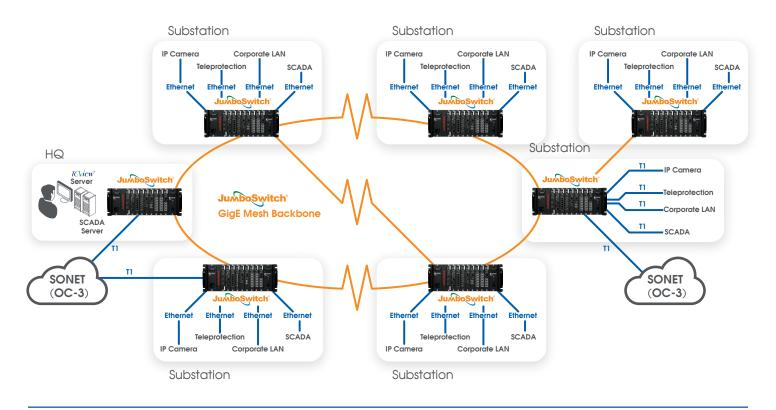
The Utility used the JumboSwitch network for a wide variety of applications including substation, SCADA, Teleprotection, Automatic Meter Reading (AMR), telecommunications, data services (including rate control), security cameras, and office LAN traffic.
