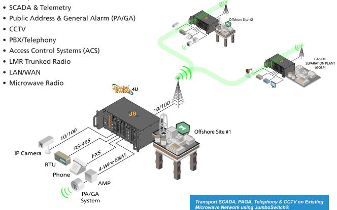
Moreover, the JumboSwitch's modular design offers users the flexibility to pay as they grow; its VoIP and TDMover-IP capability (10/100/1000 Ethernet, Fiber, T1/E1, 2/4-Wire E&M, RS-232, RS-485, etc.) gives users the ability to expand their communications networks as needed in the future.
